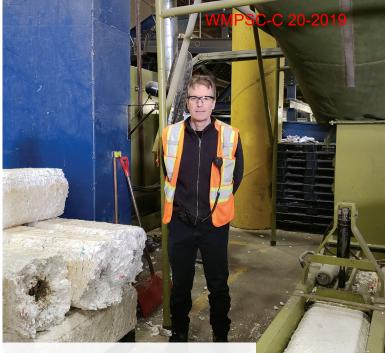
Niagara Recycling's cold-press polystyrene processing setup compacts EPS into 50-pound blocks.
