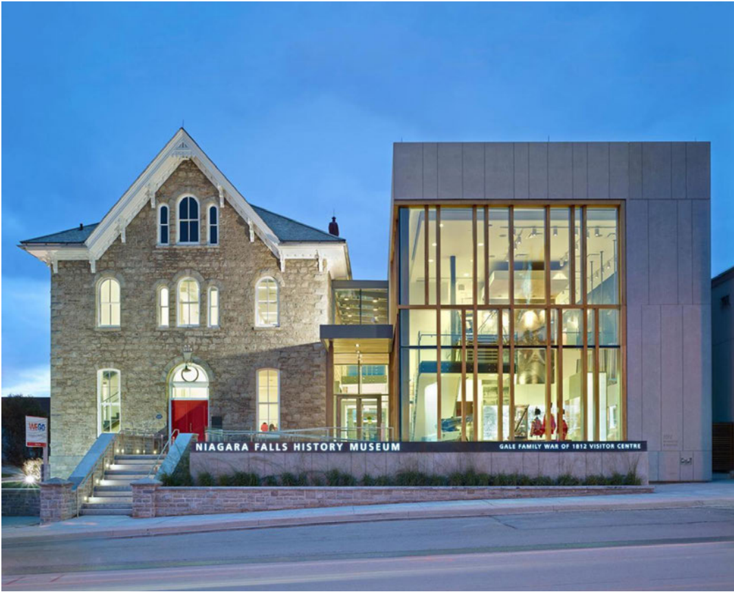
Figure 110: Additions should maintain a respectful relationship with heritage structures through the use of setbacks, the matching of datum lines, and visual breaks to ensure the dimensionality of the heritage building is legible (History Museum).
