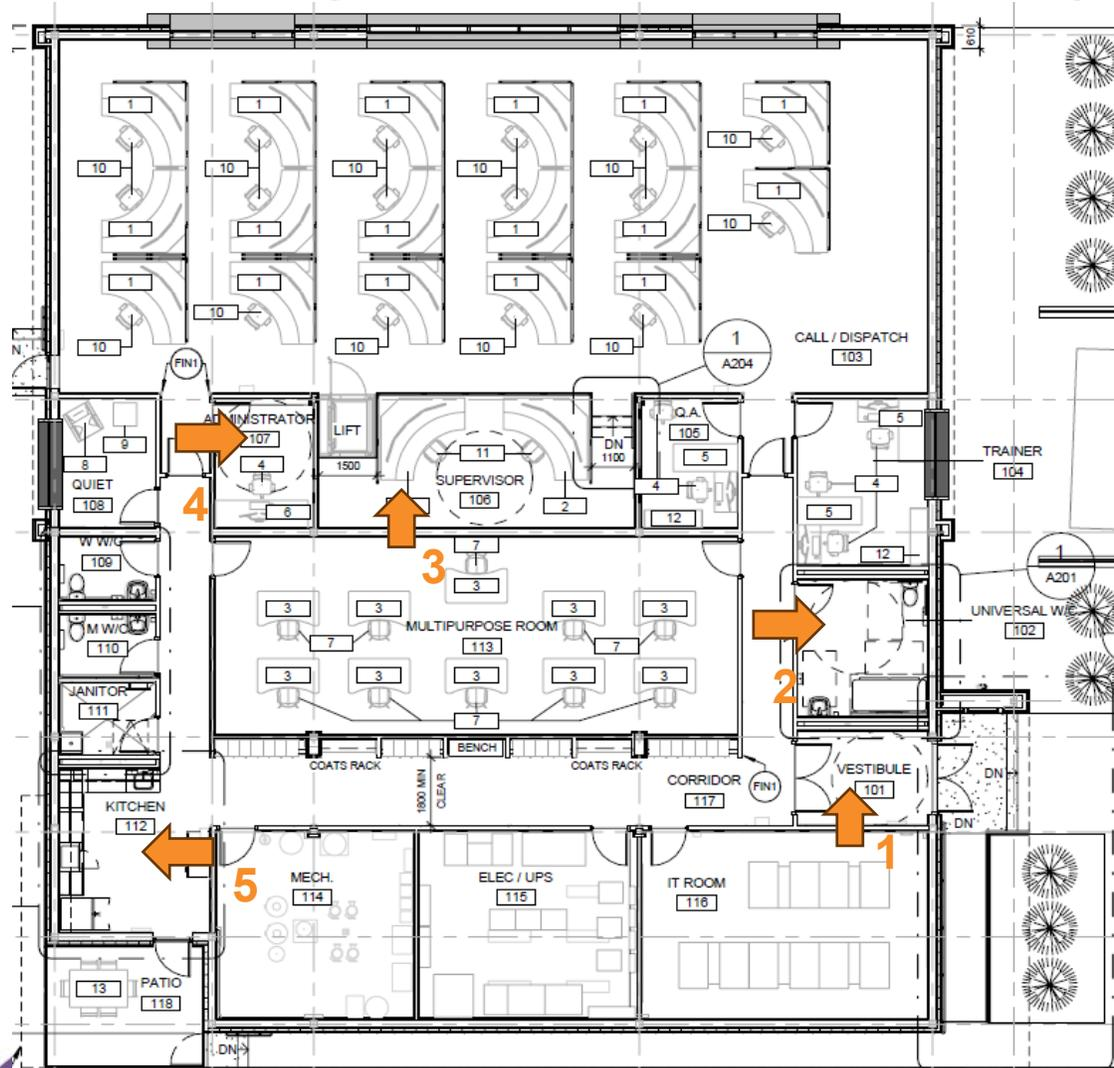
1. – main vestibule to provide clearance for Region’s Universal Design Standards of 2500mm complete with overhead door operators
