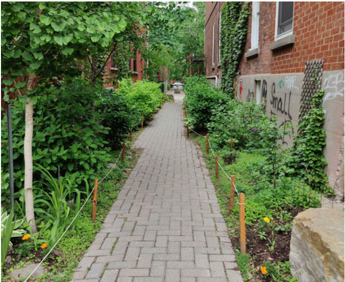
Figure 74: A pedestrian clearway width of a minimum of 2.1 metres should be accommodated within the mid-block connection.
