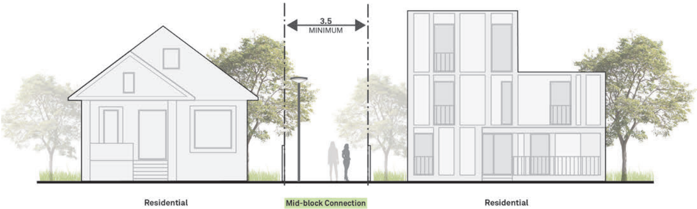
Figure 76: Residential mid-block connections should be at least 3.5 metres wide and include pedestrian-scaled lighting.
